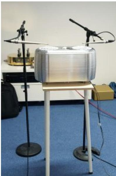
*Nearfield QC measurement setup of a monitor loudspeaker*
