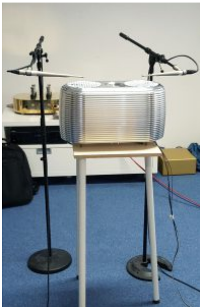
Nearfield QC measurement setup of a monitor loudspeaker
